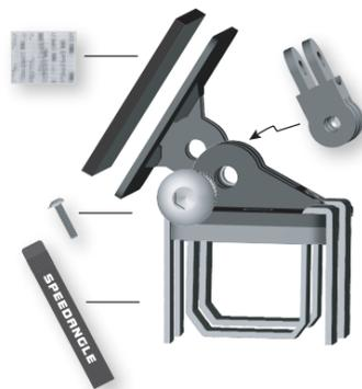
2. Adhere the two Dual Lock strips to the back of APEX.
