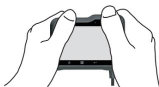
4. To remove APEX from the mount, place your fingers around its upper front. Use the base of your thumb as a pivot and pull away from the top.
